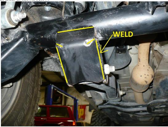
6) After welding, clean off any weld burrs and paint to the desired color to prevent corrosion.
