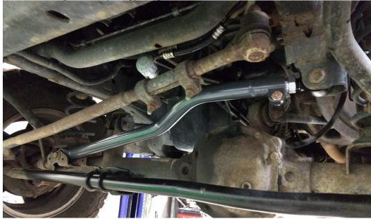
Figure 6. Correctly Installed Synergy Mfg Track Bar
