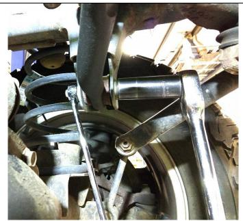
Figure 3. Removing the Track Bar from the Frame Side
