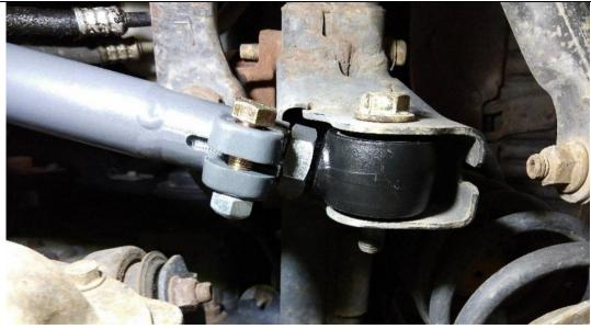
Figure 5. Synergy Mfg Track Bar Installed at the Frame
