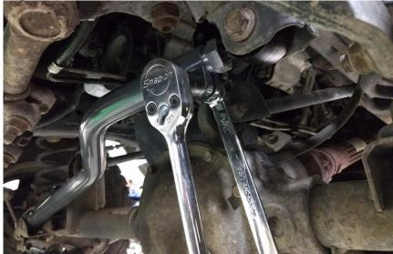
Figure 8. Tightening the pinch bolt and nut.
