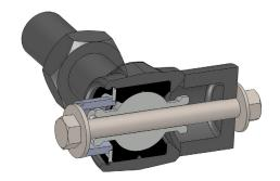
O Place the large nylon cup on the end that will not have the snap ring removed with the cupped end towards the flex eye as shown.
