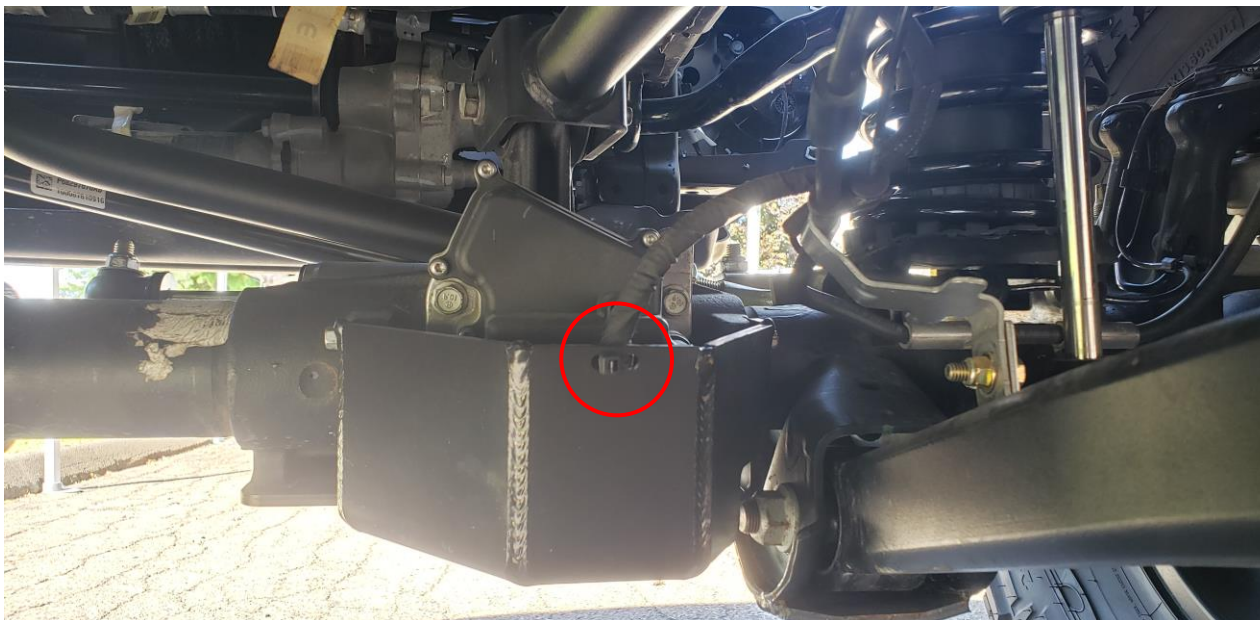
Figure 6: Rear of FAD skid plate with wiring harness secured
