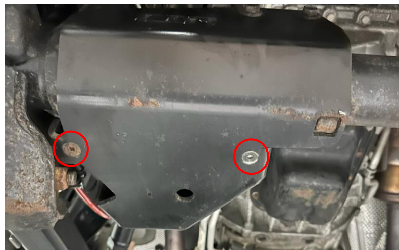
Figure 3: CAD and installation photo of FAD skid plate in position
