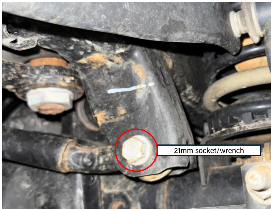
Jeep JL frame-side track bar bolt before and after removal
