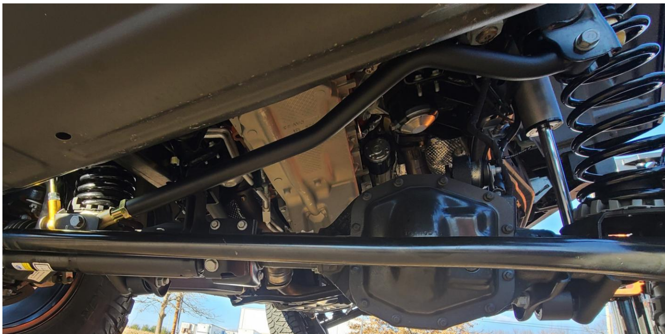
JL adjustable front track bar fully installed
