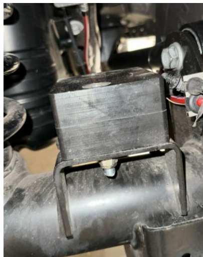
Figure 33: Bump-stops (1-2" tall stackable bump-stop options)
