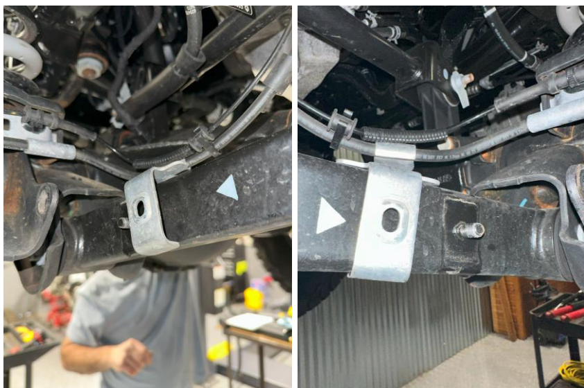
Figure 6: Front driver/passenger lower brake line mount removed
