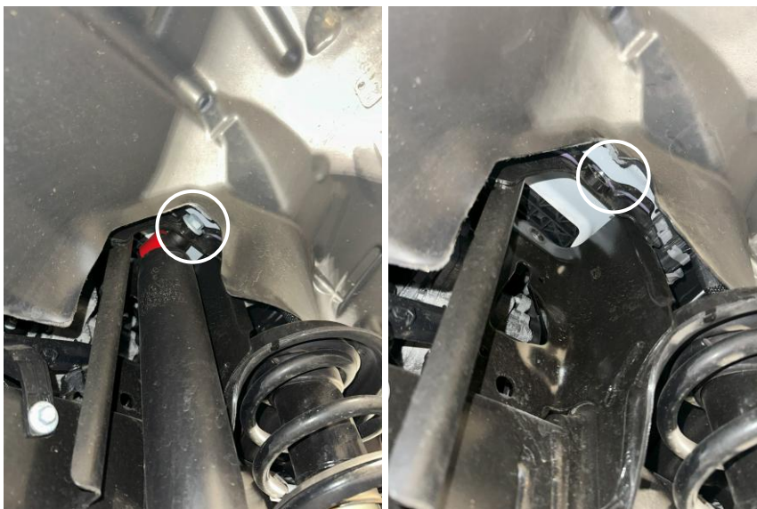
Figure 5: Front upper passenger shock bolt removed
