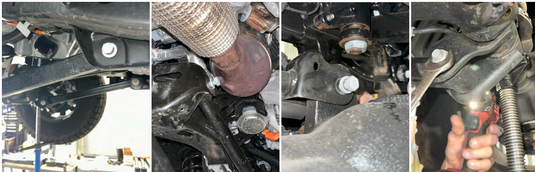
Figure 9: Lower/upper frame-side control arm bolts, and lower/upper axle-side control arm bolts
