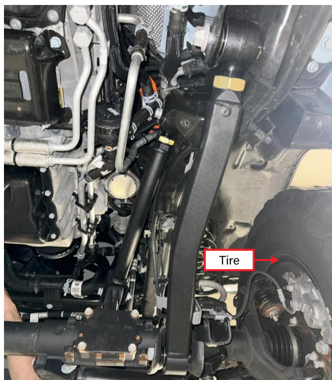
Figure 14: New passenger-side control arms installed with original hardware
