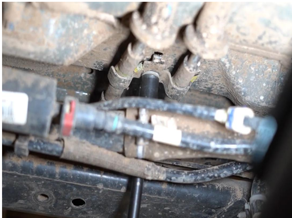
Figure 24: Emergency cable bracket dropped
