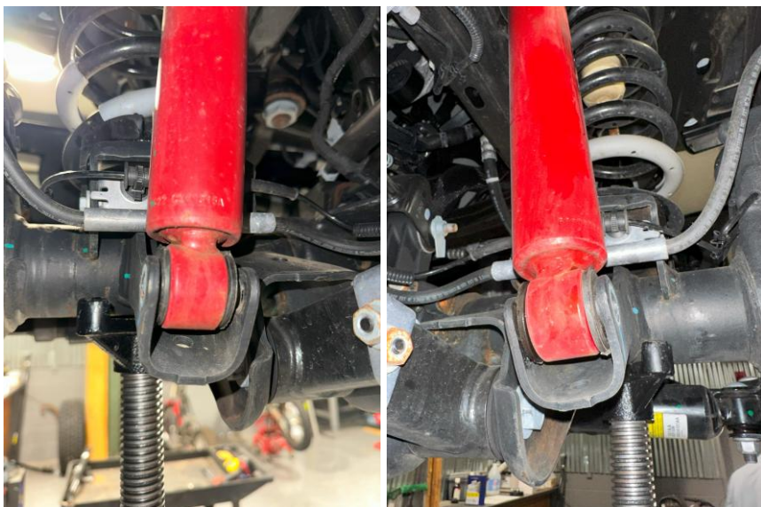
Figure 4: Front driver/passenger lower shock bolts removed
