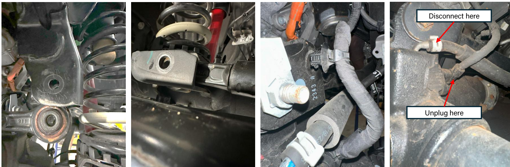
Figure 8: Front factory track bar bolts locations (left) and wiring harness/breather hose and plastic clips (right)
