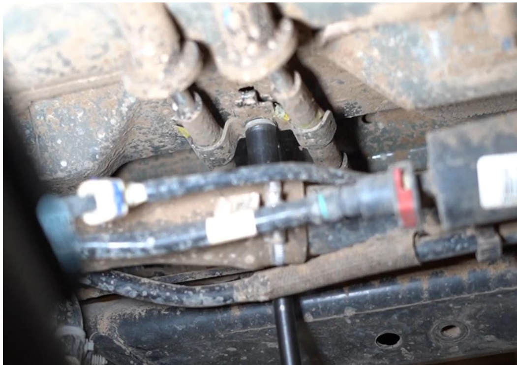
Figure 30: Emergency cable bracket tightened
