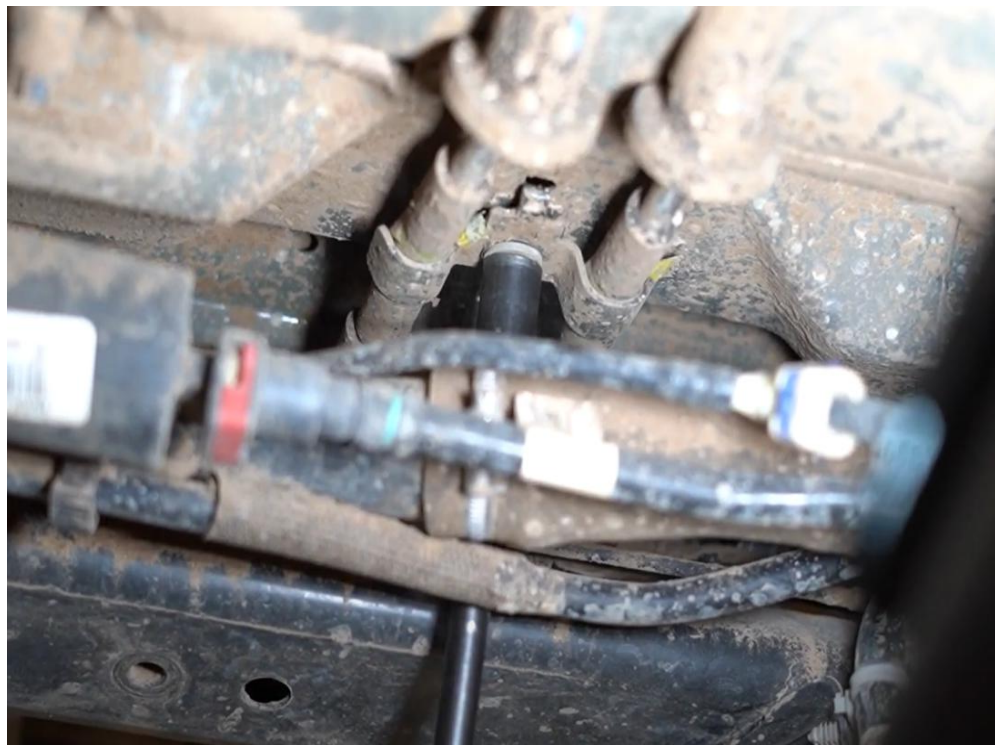
Figure 24: Emergency cable bracket dropped
