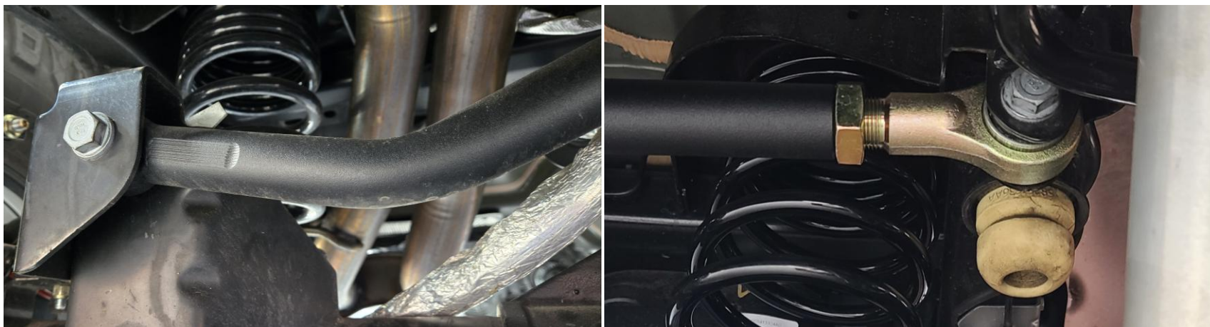
Figure 32: New rear track bar installed
