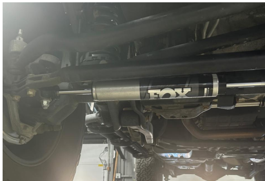
Figure 3: Steering stabilizer axle mount location (JL)
