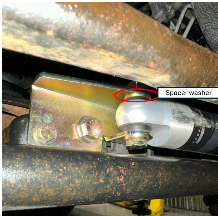
Figure 7: Steering stabilizer installed with the bolt head on the bottom of the bracket, and spacer washer installed
