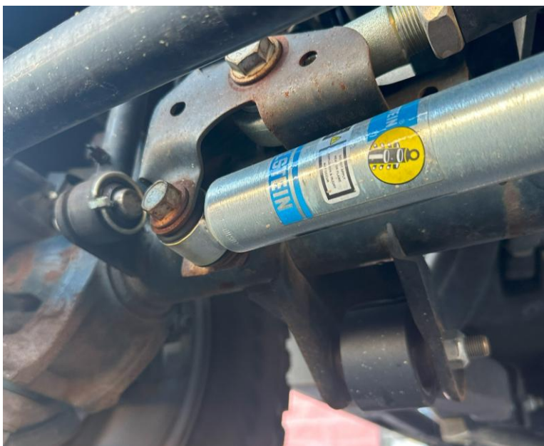
Figure 2: Steering stabilizer axle mount location (JK)
